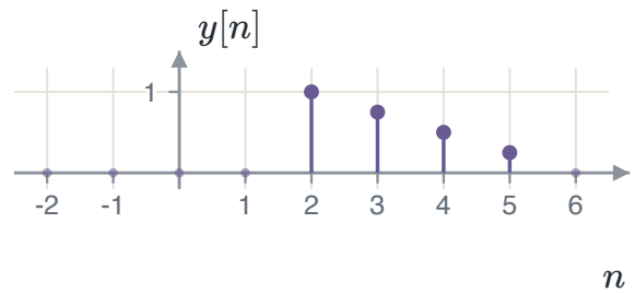
FIGURE 1.11 y[n] = x[n - 2] : every stem moves two samples right. The sample x[1] = 0.75 appears at n = 3 .
